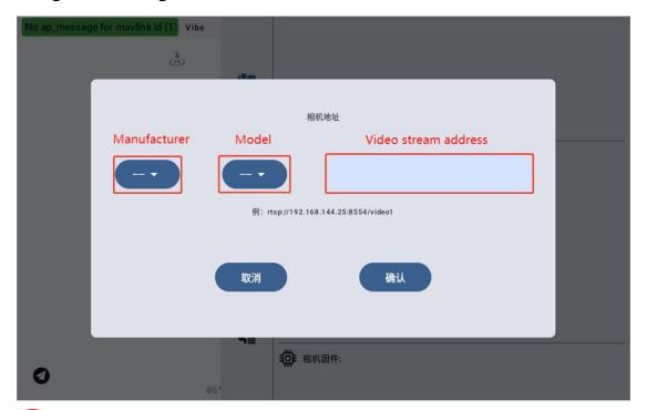
Note: When manually entering the address, ensure that punctuation marks are in English mode. If the manufacturer and the model are "——", after entering the correct video stream address, only the video will be displayed, and the camera can not be controlled. At present, the manufacturers and models only support SIYI series products.
