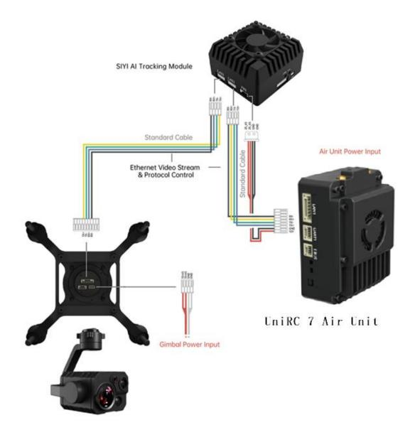
4. Refer to the diagram below to connect the SIYI gimbal camera (optical pod) to the flight controller and fuse flight controller attitude data.
