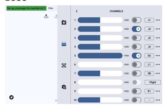
Select the target channel and click the corresponding servo forward/reverse switch to successfully set the servo direction.
