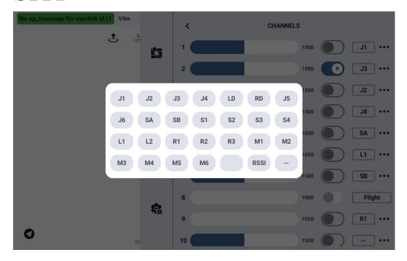
Select the target channel, click the channel mapping button, and a switch list will appear. Choose the desired switch to successfully establish the connection.
