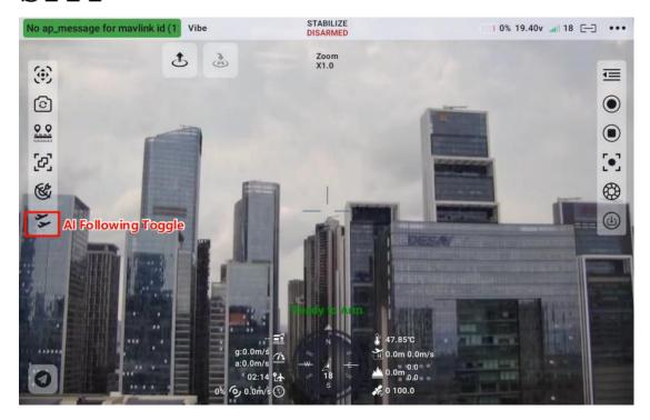
The SIYI optical pod (gimbal camera) can be connected to the airborne unit via the SIYI AI tracking module. When the airborne unit is in communication with the ground station, this application enables AI recognition, tracking, and follow-me functionality.
