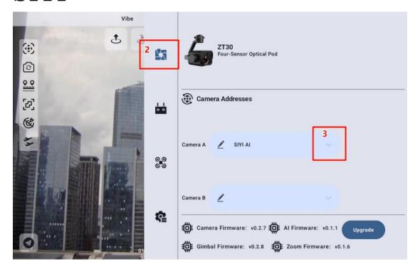
Step 3: Tap the downward triangle in the camera address bar and select the correct camera address. Alternatively, tap the pencil icon to manually enter the camera address as prompted.
