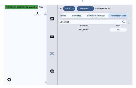
After completing the settings, write the parameters and reboot the flight controller for the changes to take effect.
