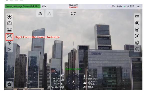
Through the UART serial port, the SIYI gimbal camera (electro-optical pod) can be controlled by the ArduPilot driver and fused with the flight control attitude data. The SIYI gimbal camera (electro-optical pod)
