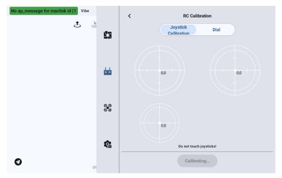
3.If the joysticks are in their natural resting position but the channel output values are not zero, it indicates that the neutral point has drifted. At this stage, do not touch the joysticks, and wait for the system to complete the neutral point calibration automatically.
