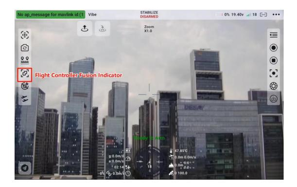
8. Switch the flight controller mode to "Guided Mode" and set the follow-me speed.
