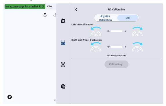
3. Follow the on-screen instructions. If the dials are at rest but the channel output value is not zero, it indicates that the neutral point has drifted.
