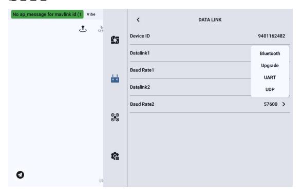
UART Serial Port: Data link communication is established via the built-in UART serial port of the ground station.
